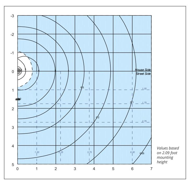
The isofootcandle values shown in the plot above are based on a mounting height of h = 2.1 feet. Grid values show multiples of mounting height. The isoilluminance contour lines are expressed in units of footcandles. The values expressed are based on the direct light from a single unit without the contribution of room reflections.
