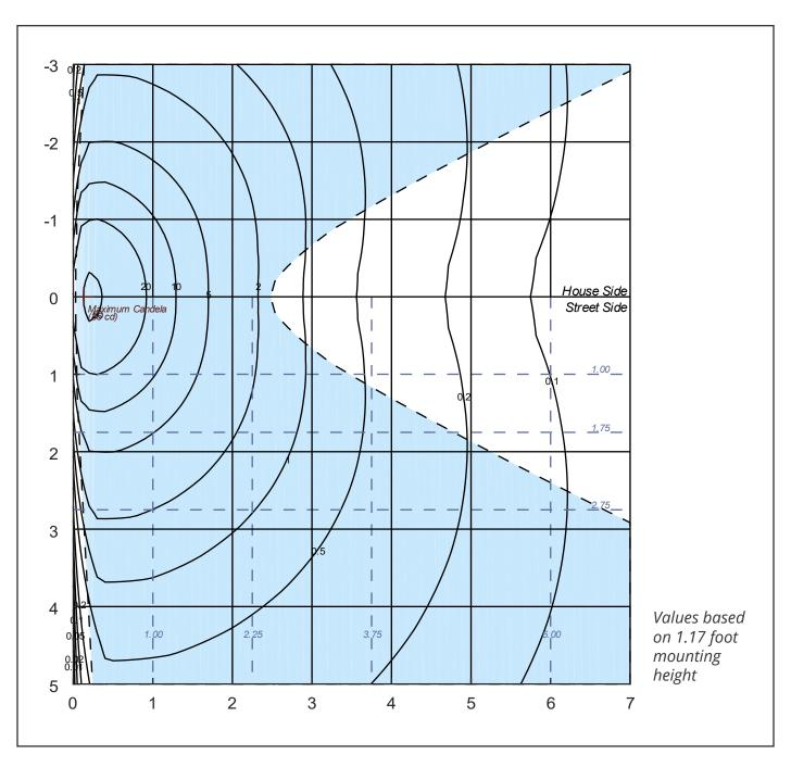
The isofootcandle values shown in the plot above are based on a mounting height of h = 1.2 feet. Grid values show multiples of mounting height. The isoilluminance contour lines are expressed in units of footcandles. The values expressed are based on the direct light from a single unit without the contribution of room reflections.
