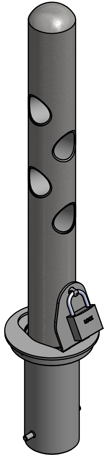
Removable Receiver with Lid (for detail, see sheet 2 of 6)
